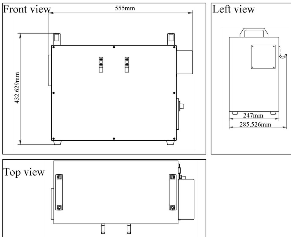
Figure 3- 2 Controller dimensions
