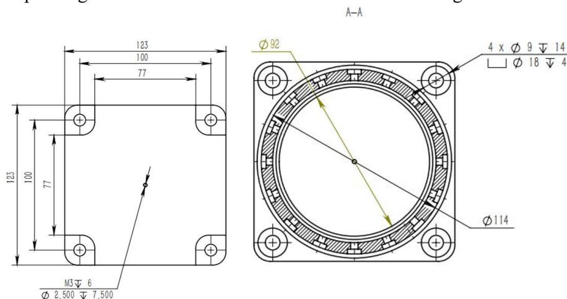
Figure 3- 1 The specific hole size
