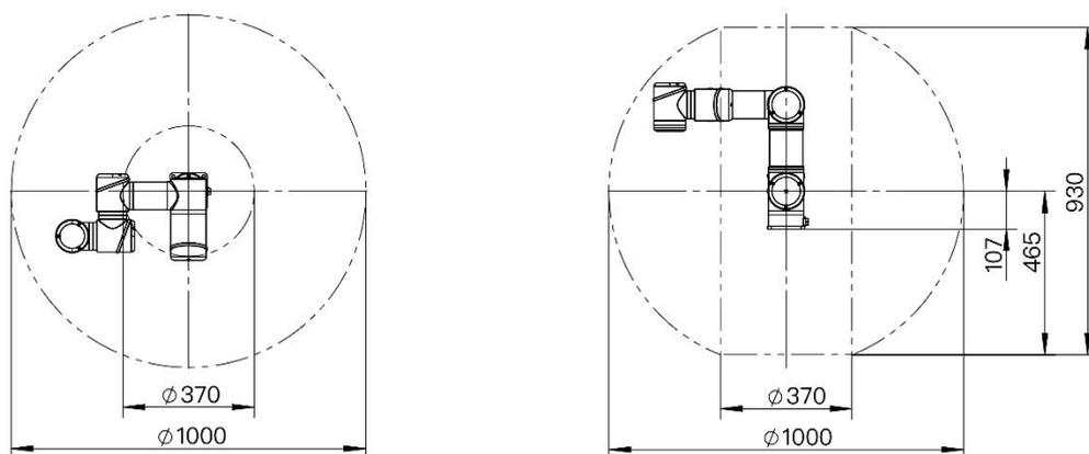
Figure 2- 3 Schematic diagram of the Panda 3 workspace
