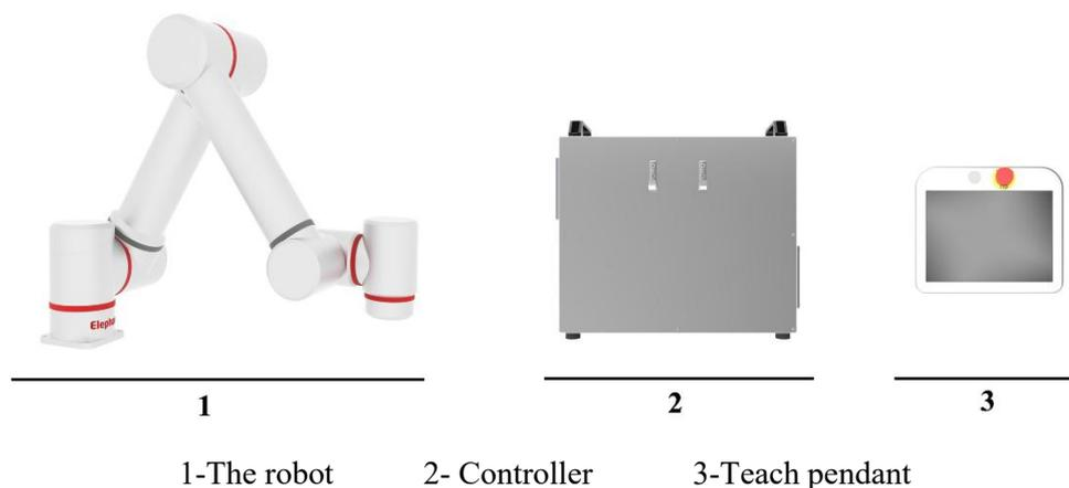
Figure 2- 1 Robot system
