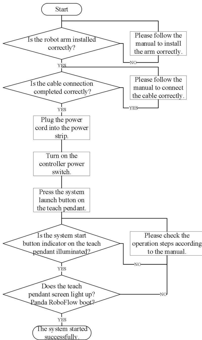
Figure 3- 5 Robot system boot flow chart
