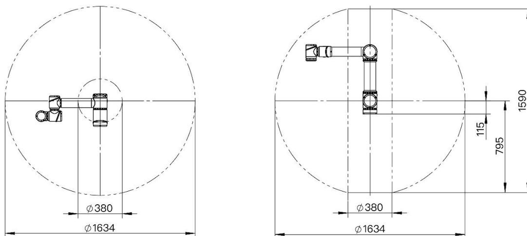
Figure 2- 4 Schematic diagram of the Panda 5 workspace
