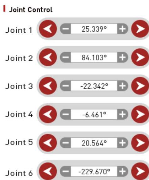
Figure 3- 9 Joint motion mode control window
